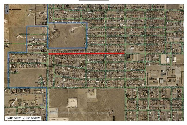
Phase 2 of W Jackson Ave was designed for construction to widen the roadway from 9<sup>th</sup> Street to 17<sup>th</sup> St adding ADA sidewalks, driveways and ramps, installing new curb and gutter all within the Cities existing right of ways. Electrical pole relocation, by Lea County Electric will take place during project, coordinated with the Contractor.
